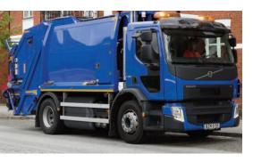
collected, compared with traditional RCV designs. Part of that is down to the HiUCV's monocoque construction, which helps to save weight. "In effect, we've taken a body and fitted wheels to it," comments Dennis Eagle managing director Kevin Else.
