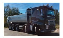
the rear. It harnesses Volvo's 'T' ride fiveleaf steel suspension on the rear bogie, instead of the usual three-leaf 'B' ride familiar in the UK. The heavier set-up is almost standard fare in Ireland – widely regarded as a 'robust' environment.
