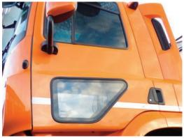
Channel's conversion involves fixing an OE spec glass panel into the CF's lower door, using a rubber seal. "We thought about bonding it, but we went for a heavy-duty glass rubber surround, not least to ensure no water ingress," explains Ades. On the inside, the lower glass pane has a bespoke GRP surround that fits within the CF door trim panel, retaining the speaker and door pocket.
