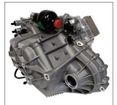
The MSYS gearbox, developed by DSD sister company Evolute Drives, is a high-torque countershaft gearbox with an innovative cone clutch mechanism. Initially a three-speed unit, it can be packaged like a conventional front-drive transaxle and promises to improve the efficiency of electric and hybrid drivetrains by 15%.
