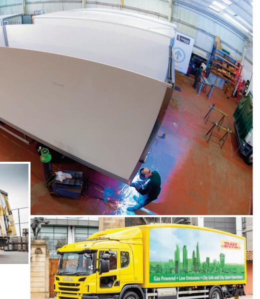
using a polypropylene welding rod.
