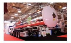
Magyar's battery-powered electric pumping system on its Eco Friendly milk collection tanker means the tractor's engine is not needed for pumping power, so there's no PTO either. The benefits are ultra-low noise, fewer emissions and fuel savings. Its lithium battery pack, mounted on the offside of the chassis, is charged by the tractor while on the move.
