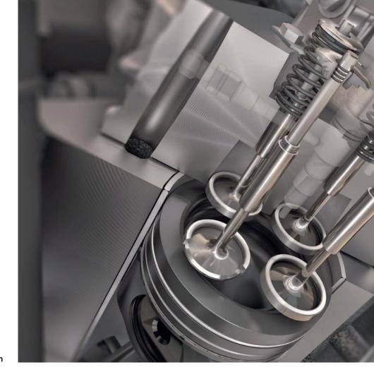
Federal-Mogul's Envirokool heavy-duty diesel steel piston will get its debut at the IAA Hanover commercial vehicle show in September. What's new is a sealed-for-life cooling chamber inside the piston crown filled with cooling oil and an inert gas, designed to prevent the coolant from oxidising. After the chamber has been charged with the oil and gas mix, it is sealed permanently with a welded plug.
