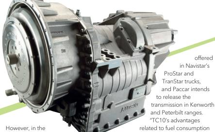
US Allison is promoting its TC10 as an alternative to manuals or conventional AMTs. Its 'blended architecture' combines a torque converter with a 10-speed twincountershaft box having multiple wet clutches to deliver constant drive. The torque-multiplying effect lets it start with a relatively tall first gear (7.40:1) while maintaining a 0.86:1 overdrive top. Allison says some have documented 5% fuel improvement with TC10-equipped tractors over current manuals or AMTs.
