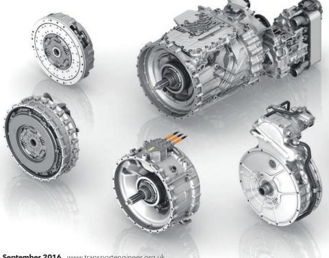
ZF's TraXon AMT can be specified with modules such as a torque converter, a DCT clutch and an electric motor
