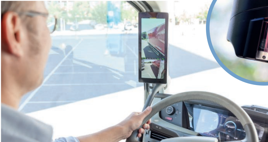
MirrorEye replaces conventional Class II and IV mirrors with HD digital cameras and interior displays
