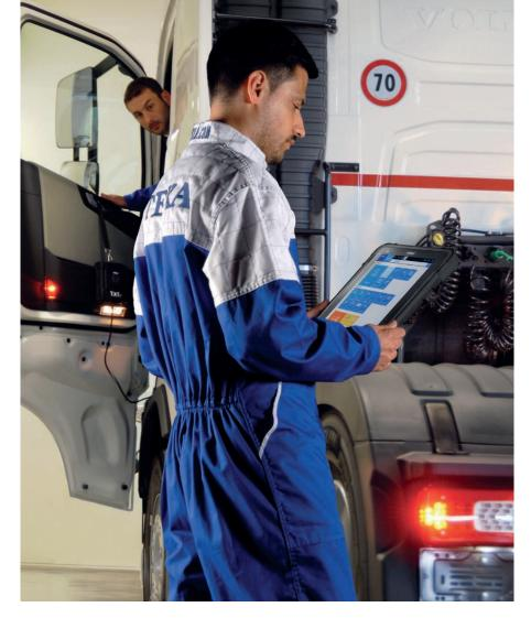
J2534 and ISO22900 define standard reprogramming interfaces, and these are required for commercial vehicles from Euro 6 onwards.
