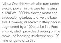
Critical to this innovative little truck's likely acceptance, however, is its PREMS (predictive range-extender management system), which harnesses GPS to determine when to fire-up the diesel and when not. For example, not in urban areas where zero emissions matter.
