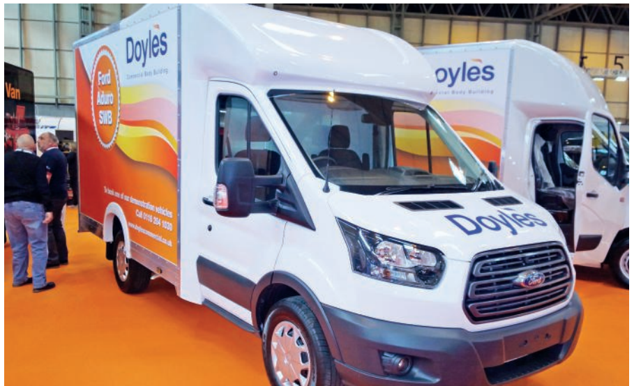
Prototype of Ford Aduro chassis cab launching next year fitted with Doyle's box body
