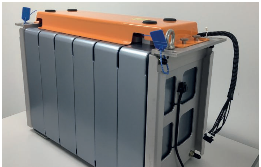
Typical single CV battery module based on 48 high-energy-density NMC cells. Up to 15 such module blocks could be used within a range-extender electric truck or bus for around 110kWh
