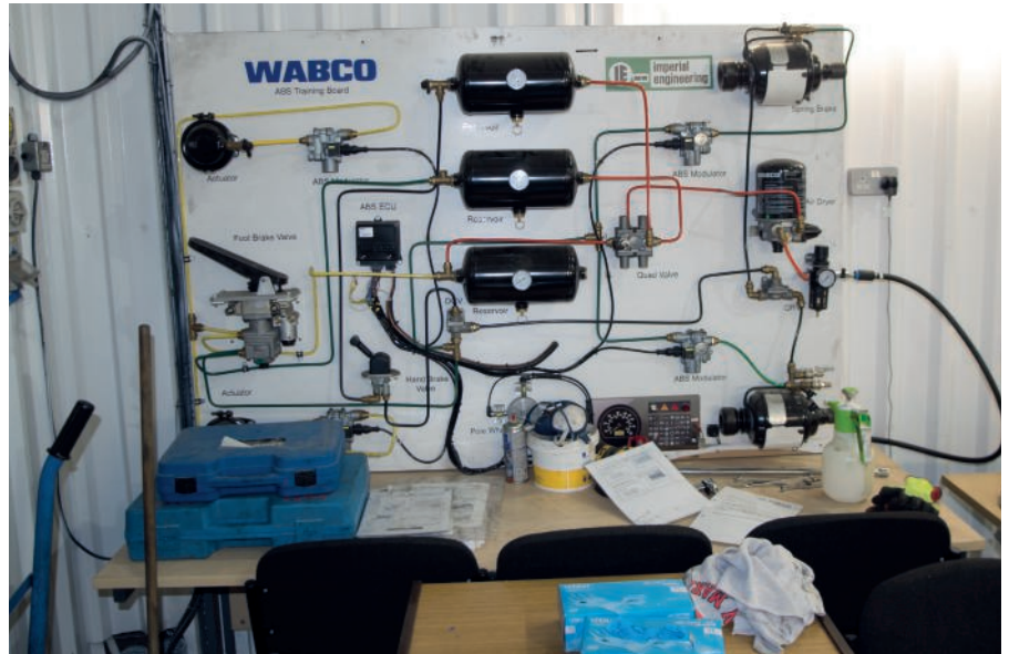
Fully functional air-brake testing board used for training at Arriva
