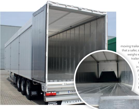
Innovations for the Next trailer include redesigned rear doors and bumpers, a light protection plate for unloading, new side protection on the chassis, lighting, a new larger platform to stand on when operating the roll-over sheet, and a reduced tare weight.
