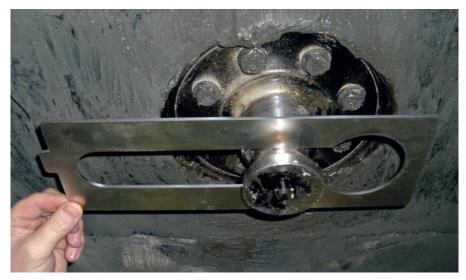
Capus wear gauge confirms kingpin girth; side tab checks pin mounting remains square
