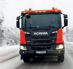
As the entire trailer is un-braked, on that long descent in Norway, at -12°C, with icy patches on the road, the instruction from Scania's professional demo driver was 'no retarder'
