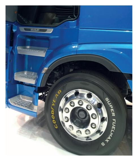
excellent mileage, superb grip and excellent wear, but also enhanced rolling resistance and so reduced fuel consumption. He claims its rolling resistance is 16% better than its predecessor. (The tyre is rated B/C on its EU tyre label for fuel efficiency.)
