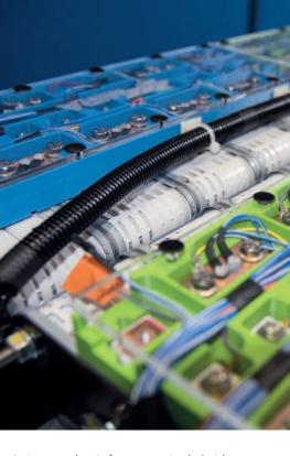
In its most basic form, a series hybrid uses an internal combustion engine (ICE)-powered generator to supply electricity direct to one or multiple traction motors. Super-capacitors or lithium-ion batteries are used to manage power demand. Plugged in and charged while the vehicle is not in use, their power is replenished on the move by regenerative braking and a generator powered by a small ICE. In theory, range can be extended up to the capacity of the fuel tank the vehicle carries.
