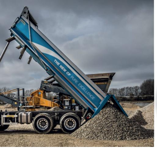
Like all new truck engines these days, the MX-11's 10.8 litres performs very well, giving a lot of bang for its buck, and with multi-torque ability. The 12-speed ZF TraXon transmission in the CF410 (402bhp) 'haulage' spec model reviewed performed well on road and off, and apart from a lower ride height than the construction version, it seemed well-suited for tipper work. Off-road in an Oxfordshire quarry, it did all that was asked of it.
