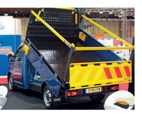
hydraulic power pack - SPX is one of the best-known manufacturers - with the control box kept in the cab and mounted on a remote control. On that topic, operators should ensure that a battery protection device is fitted. Raising and lowering the body several times a day,
