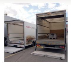
Accessing the rear (pictured above) to pick a parcel took 40 seconds in the Master and almost two minutes for the truck, with the lift having to travel much higher to reach the body floor.
