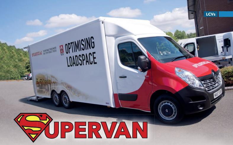
Renault Trucks has launched a 6.0-tonne Master 6x2 as an alternative to the default 7.5-tonne truck. As van chassis are becoming ever heavier - as emissions compliance tightens and specifications improve - the popular 3.5-tonne van's payload is under increasing pressure, reports Dan Gilkes
