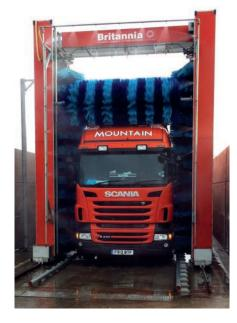
the front of the vehicle; he or she drives forward and the sides are cleaned; then the vehicle is stopped and the rollover wash cleans the rear.
