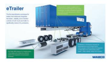
state of the battery and controls the e-drive to perform the recuperation and propulsion processes. Acceleration or deceleration requests are transmitted from truck to trailer via ISO communication to further extend the integration of Trailer EBS in the overall vehicle control system.
