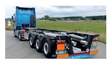
Triplex, weighing in at 4,480kg in its basic form. Offering a gross tare weight of 41,000kg and a fifth-wheel load of 14,000kg, the chassis is intended to transport 20-, 30-, 40- and 45ft ISO containers as well as 40- and 45ft Highcube containers. It features
