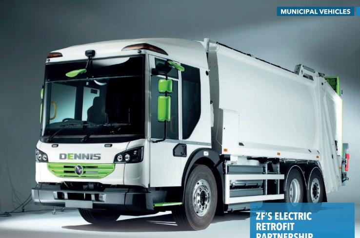
The project, which wound up in March 2018, has produced five pre-production vehicles, now out on customer testing. Three units have been made of a 'light' 16t gvw 4x2 model that can carry 1.5t more than a standard 18-tonner, thanks to its new body, and powered by a 4.5-l engine (a smaller production diesel isn't commercially available). A second variant is a CNG-powered 26-tonner vehicle that is targeted to reduce CO<sub>2</sub> by 15%.
