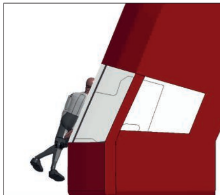
Future buses will have a more sloped windscreen to try to deflect pedestrians
