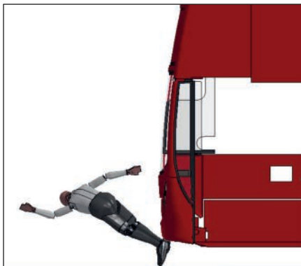
In a collision, current buses tend to push an average pedestrian down towards the ground
