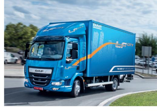
or 170bhp, it is equipped with a fivespeed Eaton manual transmission. Smaller than the 4.5-litre and 6.7-litre diesels installed in other LF models, the 3.8-litre achieves Euro VI emissions compliance by relying solely on selective catalytic reduction (SCR). Exhaust gas recirculation (EGR) is not fitted, which helps save weight.
