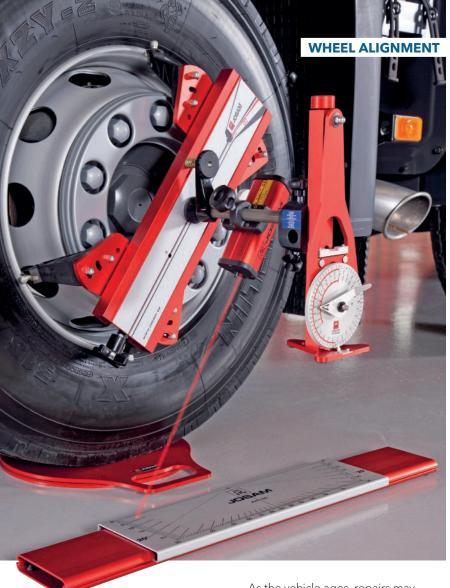
are positioned perpendicular to the chassis centreline, and that the axles themselves are centred correctly, parallel to one another and to the ground.
