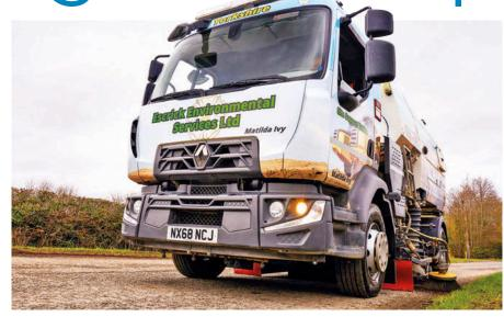
VE651 is fitted with a pair of 22kW onboard chargers which allow the battery pack to be fully replenished in four or five hours, the manufacturer contends. It can be supplied with 16A, 32A or 63A charging cables and it can be charged from a 415V AC three-phase socket. The pack is guaranteed for five years and should cope with 3,000 charging cycles.
