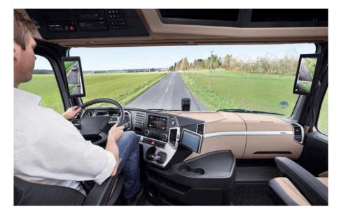
mirrors. The remit was to reduce damage costs and insurance claims caused by the mirror, particularly on the nearside.
