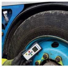
tread depth is 12-14mm). The technicians follow a pattern specific to each tread type, which is also available on their tablet. The operation is usually carried out on loose tyres back at the hub.
