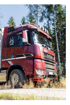
Danfoss supplies an electric motor to Sisu to boost the 616bhp of its 15.6-litre Mercedes diesel up to a maximum combined output of around 888bhp, making the 900 Polar+ easily the world's most powerful road-going truck
