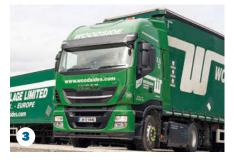
Cursor 13 NP engine and automated transmissions. Range varies from 570km on CNG to 1,600km on LNG. There is also a low-chassis LNG-only 4x2 with the same cab options, but range constrained to 750km on LNG-only. The 6x2 option has the 454bhp Cursor 13 NP engine plus automated 'box and a 750km range on LNG only. There is no SCR or PM filter.
