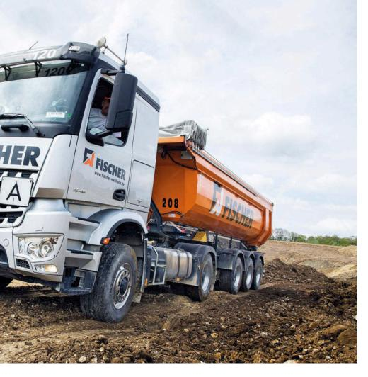
with lightweight cast suspension and an axle optimised for 44-tonne work," he says. Like Handy and Moon, Comer points to the chassis packaging benefits such axles can bring. "If we want to fit additional equipment - a blower for example - on a 4.0m-wheelbase chassis, then we can take advantage of up to 970mm of free space on the right-hand side," he says. Extra room is especially useful if the truck is running on a gaseous fuel, and needs to
