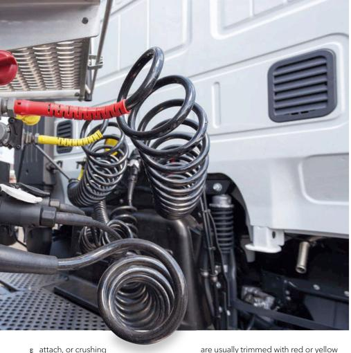
of the pipe itself, which can lead to a slow release of air, and can cause brake dragging and overheating."
