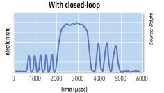
Up to nine injection events per cycle Smaller pilot and post injections 2mg/5mg Smaller separation 100µsec
