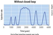
Up to five injection events per cycle Pilot/post injections 4mg/10mg Separation 300µsec
