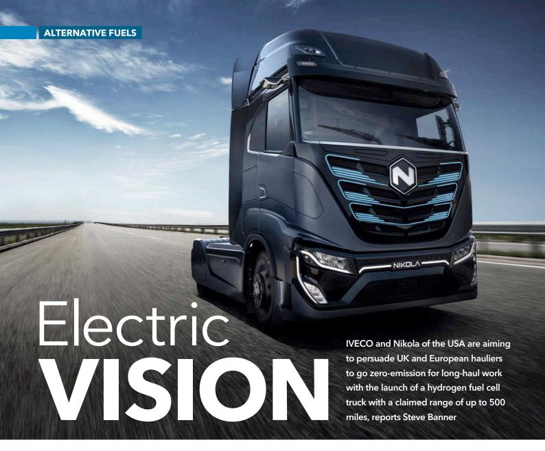
he Nikola Tre is based around IVECO's S-Way tractor unit, with Phoenix, Arizona-based Nikola providing the fuel cell technology. Around 40kg to 80kg of hydrogen is held in high-pressure carbon-fibre tanks mounted between the truck's chassis rails which can be refilled in around 15 minutes, say the manufacturers. Maximum power output is 300kW (402bhp).
