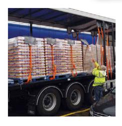
a load. A high LC value does not automatically mean a high STF, and vice versa." He adds that a thinner polyester webbing can achieve higher tension forces than a thicker one with the same tensioning device.
