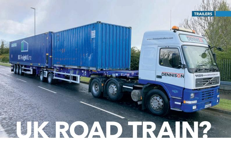
he key element in trailer manufacturer Dennison's road train design is a two-axle link trailer that sits between the tractor and a standard 13.6m-long semi-trailer. It has manufactured more than 800 of them since it launched the design in 2008, according to Stuart Wardlaw, a transport consultant at Logistics Fleet Management Support, which is representing the firm. He says that 25.25s are operated in Scandinavia and continental Europe.
