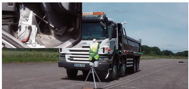
The system detects the cyclist in the danger zone (pic 1) and automatically stops the truck if it is on a collision course (pic 2), allowing the cyclist to pass unharmed
