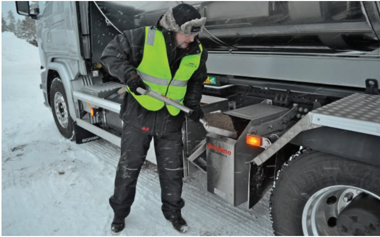
Automatic sanding ahead of the drive wheels can make all the difference to traction setting off
