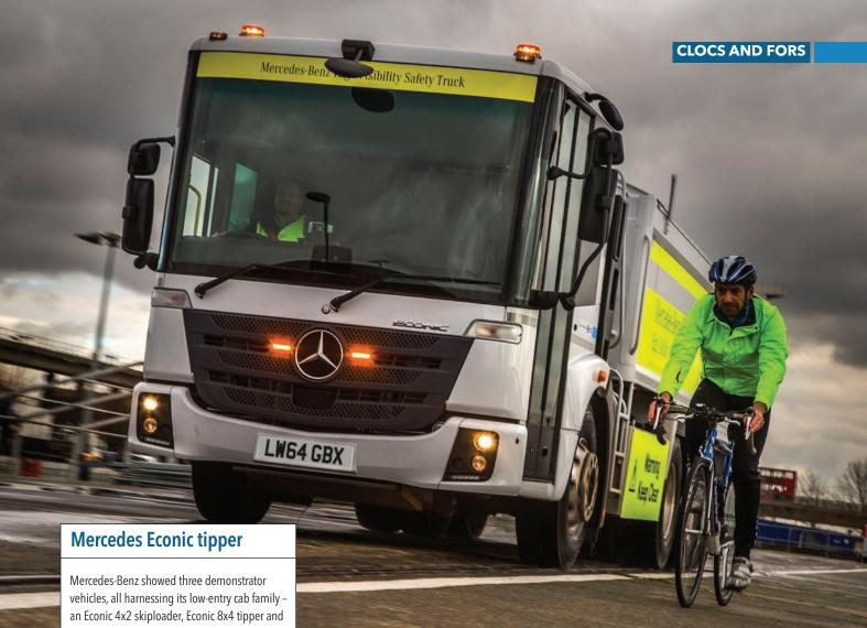
Mercedes-Benz showed three demonstrator vehicles, all harnessing its low-entry cab family – an Econic 4x2 skiploader, Econic 8x4 tipper and an Econic 6x2 cement mixer. It was a convincing act: while most others are working hard to adapt their trucks for safer working in urban environments, the Econic has 16 years' history, and not just with RCVs.
