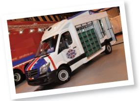
on a Mercedes Sprinter with lowered Al-Ko Kober chassis plus an aerodynamic lightweight body, using ultra-thin insulated panels. Curtis explained that the vehicle is highly configurable, pointing to a bus-style articulating side door, externally accessed shutter racking and a rear ramp door for impressive loading bay compatibility.
