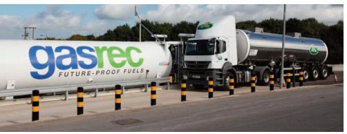
Westport spark-ignition Euro 6 CNG-powered engine, delivering 320bhp and 1,356Nm maximum torque, yet again mated to a six-speed Allison auto. Truck options are 19-tonne 4x2 or 19.5—26 tonne 6x2 rigids.
