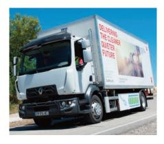
electric truck with a range extender, its electric motor (103kW) runs with a diesel unit delivering 132kW. It's an interesting reversal of the usual logic that sees the conventional engine as the main event, helped by an electric motor with less clout.
